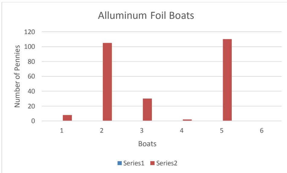
**Analysis:** During this experiment five boats were tested. The first boat was done without any research and could only hold 8 pennies until it took in water. For the second boat, research told that the boat would hold more pennies if the boat had straight edges. So this boat had four straight
